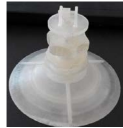
Fig. 14.The prototype of new suction disc with glue cavity by 3D printer
